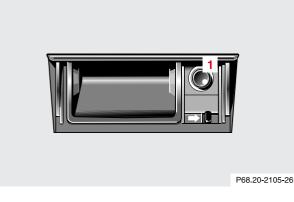
Turn electronic key in steering lock to position 1 or 2. Push in lighter (1); it will pop out automatically when hot.
